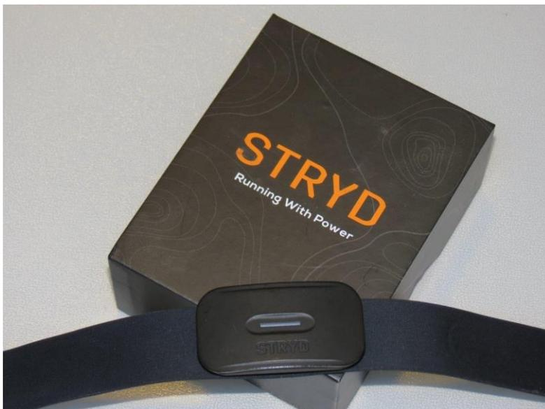
The Stryd Pioneer is attached to a chest band that also measures your heart rate (photo). You can easily connect it to your running watch or smart phone. Sensors measure the acceleration of
