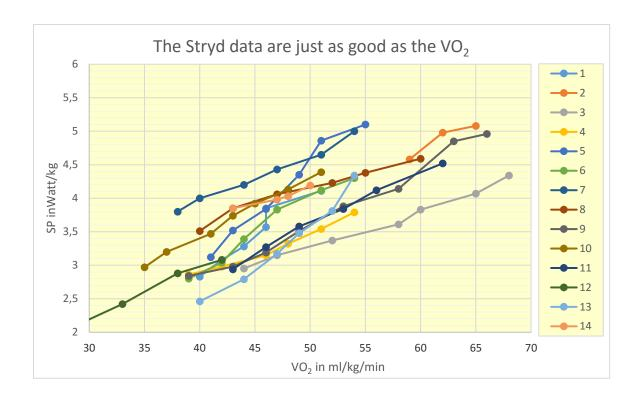
Based on the comparable results, we concluded that in general the Stryd data are just as good as the  $VO_2$ . This means that runners can now use their daily power data as an alternative to the once-a-year laboratory measurement of their  $VO_2$ .
