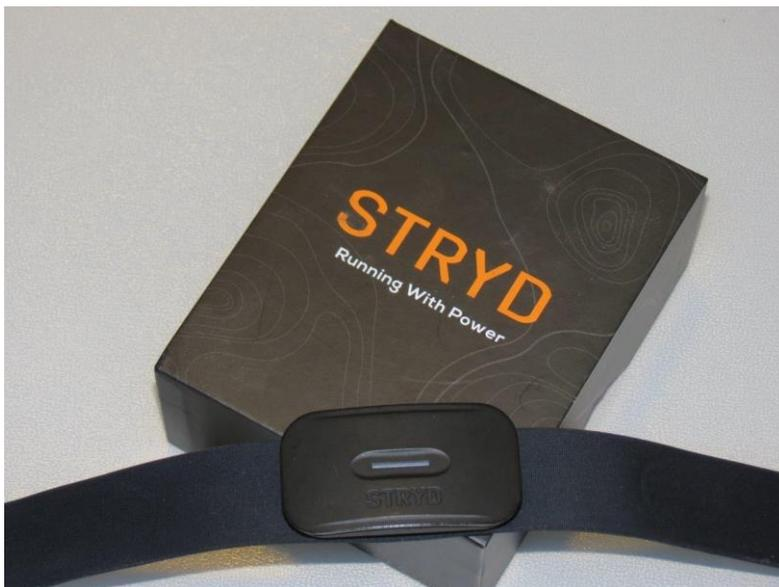
The Stryd Pioneer is attached to a chest band that also measures your heart rate (photo). You can easily connect it to your running watch or smart phone. Sensors measure the acceleration of your body in 3 directions: horizontal, vertical and lateral. Obviously, in running you would want to limit the vertical and lateral movements as they increase the energy cost and do not contribute to the forward movement!
